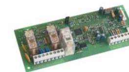
J400-EXT Extinguisher module with microprocessor control
